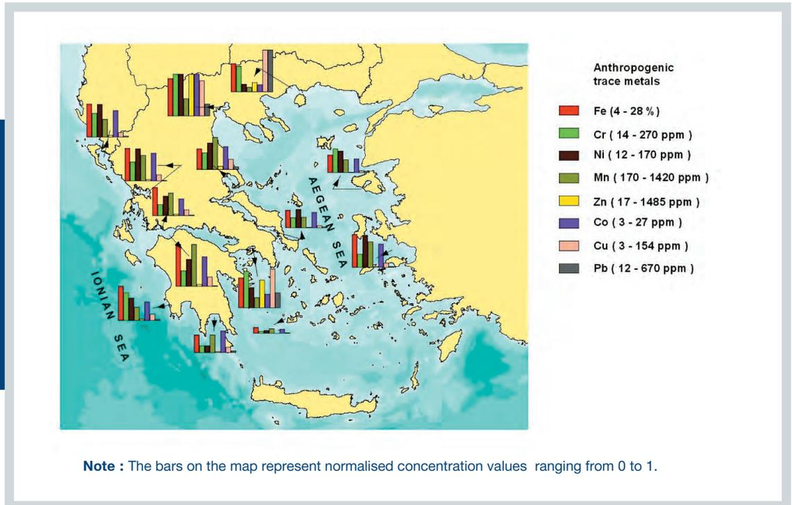
**Figure IV. 27:** Stations 1, 2 correspond to unaffected sediments from the Fe-Ni smelting plant. The enrichment of stations 3 to 6 in heavy metals is obvious.
